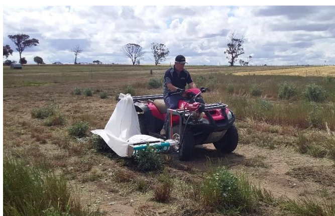
Figure 16: An earlier prototype of the harvesting machine, with the tea-harvester mounted on a quad bike.
